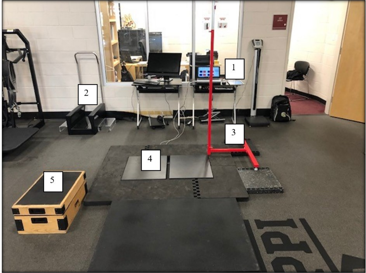
Figure 3.8 Experimental jump set-up: (1) Laptop running ForceDecks Software, (2) Adidas Foot Scanner, (3) Vertec Jump System, (4) Dual Force Plates, and (5) Drop Jump Box was positioned on platform adjacent to force plates during testing.
